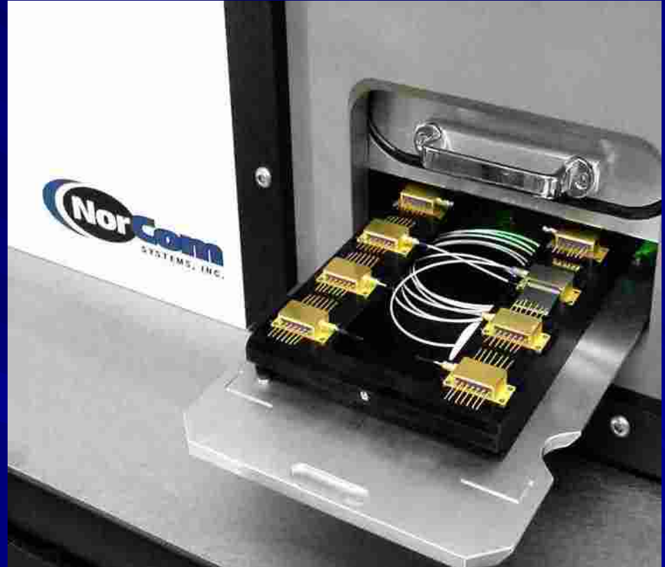
Operator places tray into system and closes chamber door.
