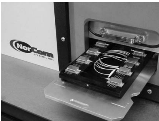
Fig. 5 Tray of devices loaded into LT-5500. Other system models are configured for semiconductor, MEMS and board level leak testing.
