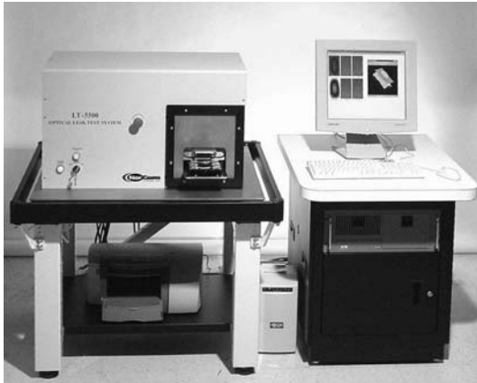
Fig. 4. The LT-5500 Optical Leak Test system showing the test chamber with the access door open, control console, printer and UPS. The digital holography camera is located above the test chamber. This system is designed specifically for leak testing optoelectronic devices in carrier trays up to 288mm in length. Gross and fine leak testing is automatic.
