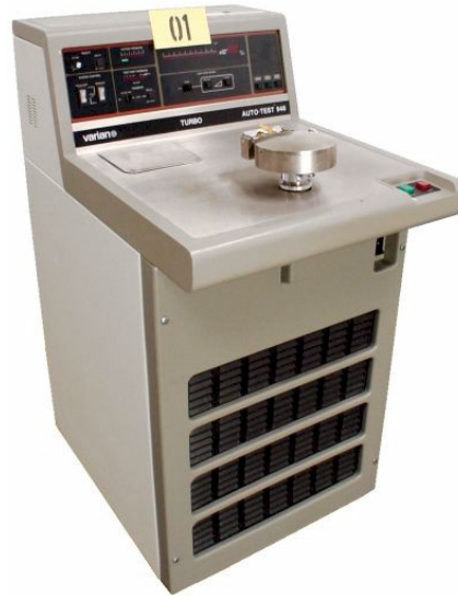
Helium Leak Detector (Varian Inc)
